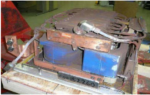
Figure 3.14. Failure of a replacement reactor module at Henday.
