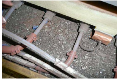
Figure 3.14. Failure of a replacement reactor module at Henday.
