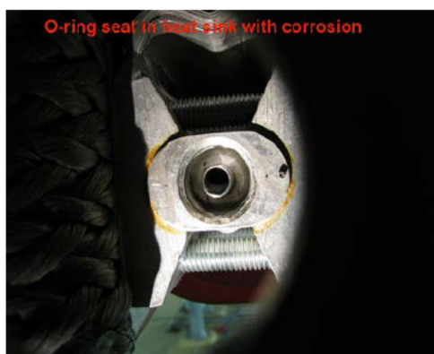
Figure 4.6. Corrosion of aluminum heatsink.
