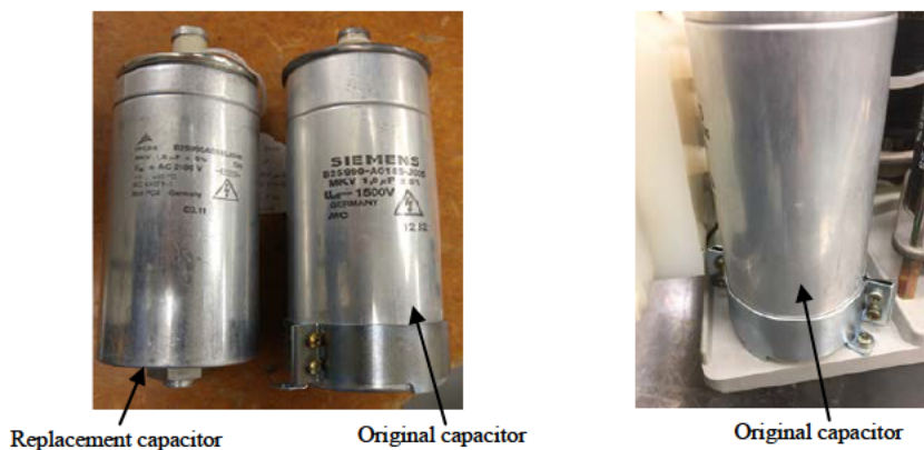
Figure 3.16. Comparison of original and possible replacement grading capacitors.
