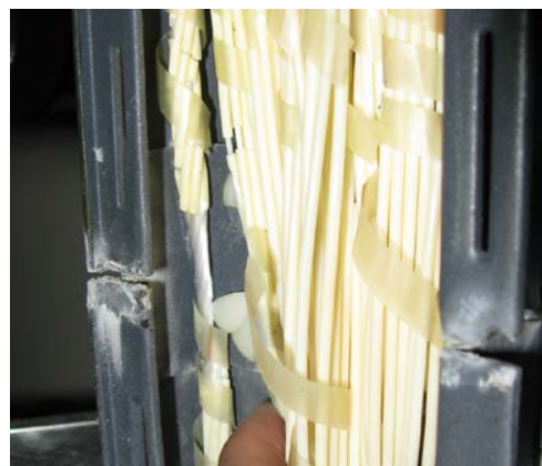
Figure 3.10(a). Severely deteriorated LG insulation jackets at Henday.
