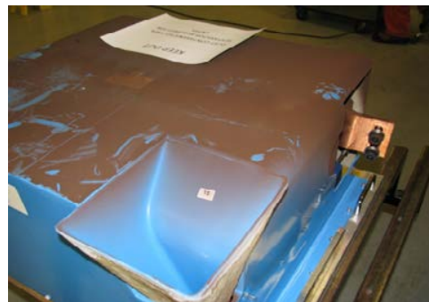
Figure 3.15. Failure of a replacement reactor module at Dorsey.
