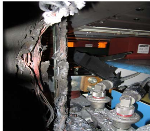
Figure 3.4. Damage caused by flashover due to a water leak in VG32 at Henday on December 04, 2011.
