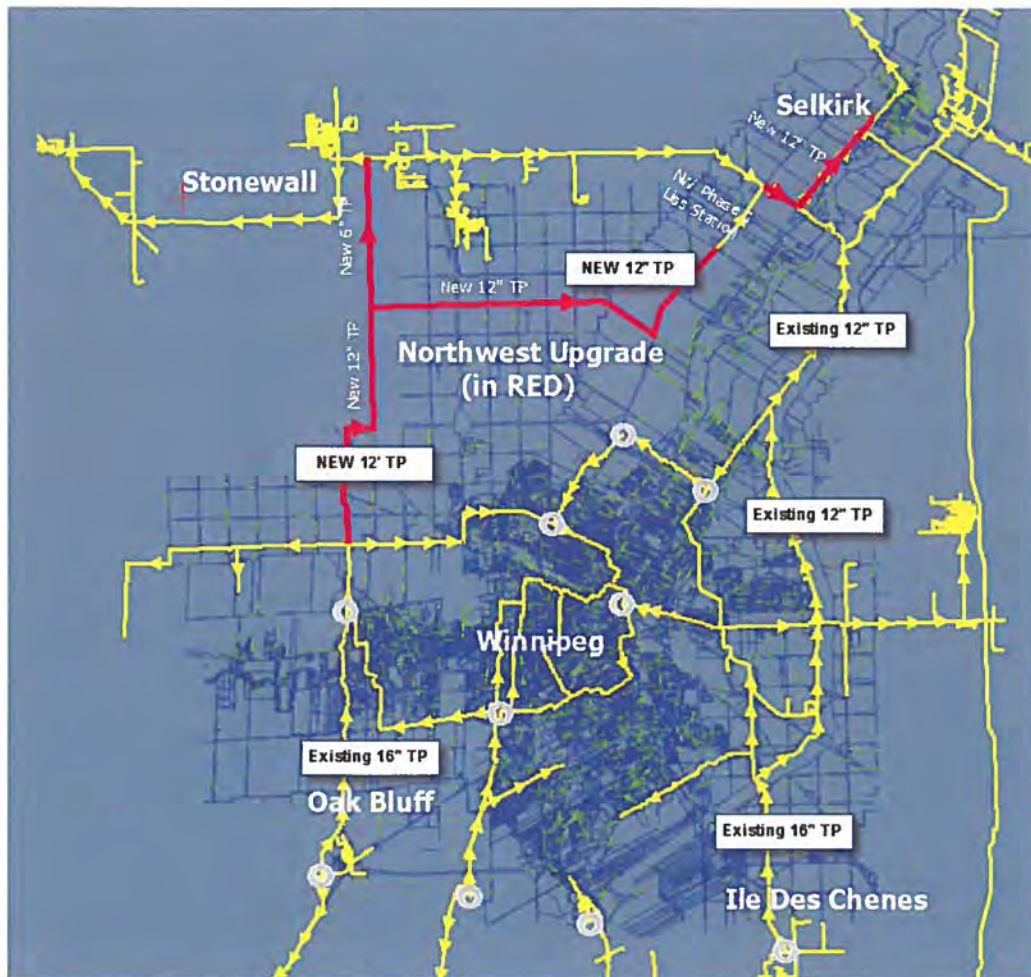
Figure ES:1 – Proposed Winnipeg Northwest Upgrade (shown in RED) Winnipeg Transmission Pressure (TP) Network
