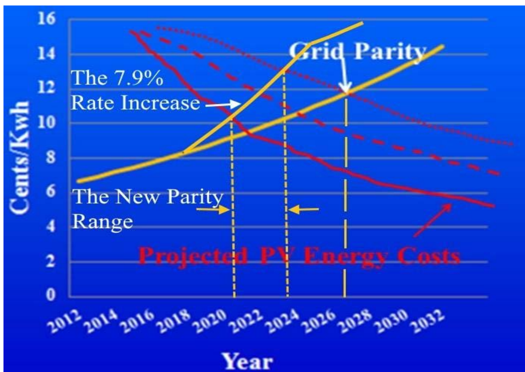
Figure 2. Impact of the 7.9% electric rate increase on grid parity and the lowering cost of solar power
