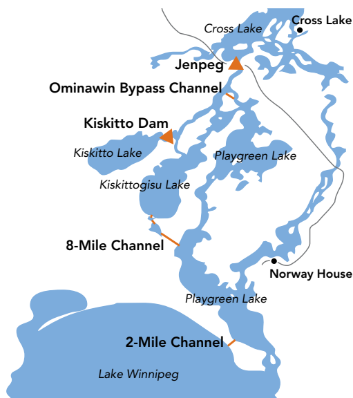
The Lake Winnipeg Regulation project involved increasing the outflow capacity of Lake Winnipeg – for both flood/drought relief and hydro-electric production – by excavating a new outlet at the north end of the Lake and construction of a control structure and generating station downstream of the outlet on the Nelson River at Jenpeg. Outflows from the Lake are controlled to keep the Lake from going too low or too high, generally within a four-foot limit.
