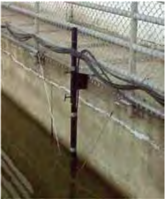
Hydroacoustic fish transducers were mounted on the upstream face of the powerhouse to estimate the number and size of fish passing through the Great Falls powerhouse.
