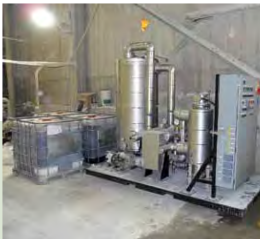
Manitoba Hydro commissioned the Mobile Burn Test Unit (MBTU), a new technology designed and built to specifically meet the requirements of the Bioenergy Optimization program. The MBTU heats and pumps pyrolysis oil to the burner at correct temperature, pressure and flow rates.
